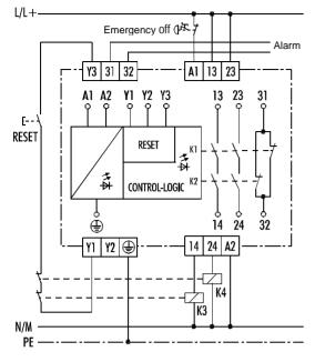
One-channel monitoring of an emergency-off momentary contact switch up to category 2 acc. to EN 954-1. Manual start is achieved through the RESET momentary contact
